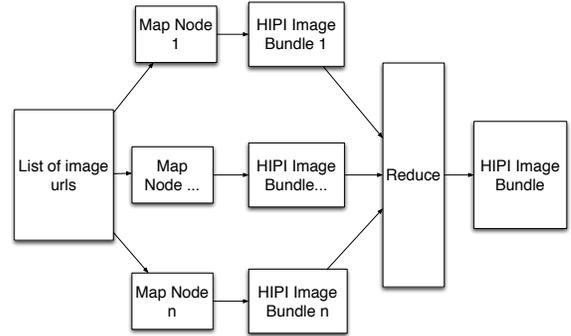
Figure 6: A demonstration of the parallelization in the Downloader application. The task of downloading the list of images urls is split amongst n map tasks. Each mapper creates a HIPI Image Bundle, which is merged into one large HIPI Image Bundle in the Reduce phase
