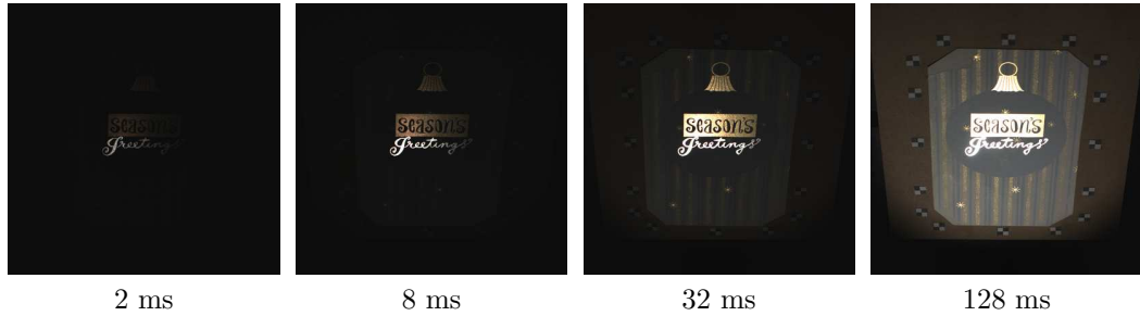
Figure 3.2: Images of the Season’s Greetings SVBRDF at different shutter speeds for a fixed camera and light position. These images are combined to form a high-dynamic-range (HDR) image that records the amount of radiance reflected into the camera at each surface position using the technique of Debevec et al. [25].
