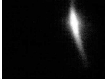
Figure 2.5: An image of brushed aluminum reflecting light from a small source. Notice the elliptical highlight that results from uneven scattering along and against the orientation of the surface’s microcylinders. Figure reproduced from [109].
